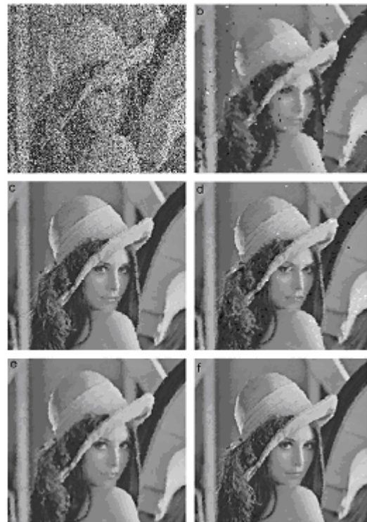
Figure 2. Image restoration results: (a) Lena image corrupted with 50% impulse noise (b) SMF (c) AMF (d) CD-SMF (e) IDFRWRIN (f) Proposed
