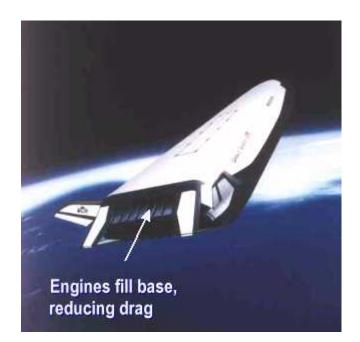
Illustration of aerospike nozzles installed on the X-33 [from Rocketdyne, 1999]
