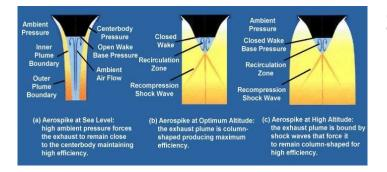
Aerospike nozzle behavior during flight [from Rocketdyne, 1999]
