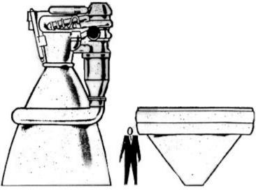
Size comparison of a bell and a plug nozzle [from Berman and Crimp, 1961]
