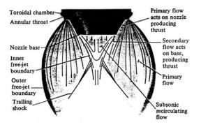
Example of an aerospike nozzle with a subsonic, recirculating flow [from Hill and Peterson, 1992]
