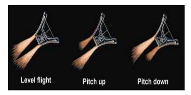
Aerospike thrust vectoring control [from Rocketdyne, 1999]
