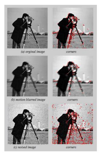
fig(12) More examples for detecting corners in : (a) normal image (b) blurred image (c) noised image
