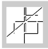
fig(9) Binary image represents the high gradient pixels ,0(white):no gradient ,1(black):high gradient
