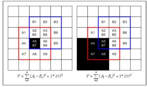
fig(1) Measuring the intensity Variation by using  $3 \times 3$  window
