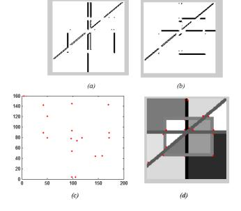
fig(10) (a) the pixels with horizontal gradient x-direction (b) the pixels with vertical gradient y-direction (c) distribution of corner points (d) localization of corners detected as final result
