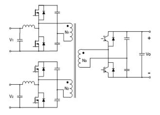
Figure 5: Bidirectional dc/dc converter triple half-bridge
