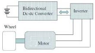
Figure 1: Bidirectional converter
