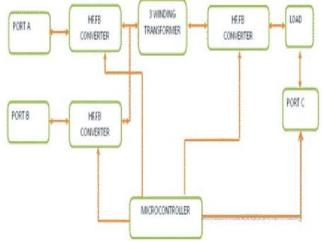
Figure 4: Multi-port converter's Block diagram
