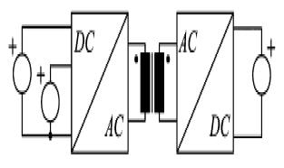
Figure 2: DC-DC converter with transformer
