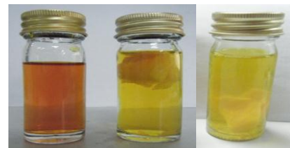
Decolourization of Tartrazine on 3 rd day (middle), 5 th day (right) and control (left)
