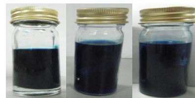
Decolourization of Brilliant Blue FCF on 3 rd day (middle), 5 th day (right) and control (left)
