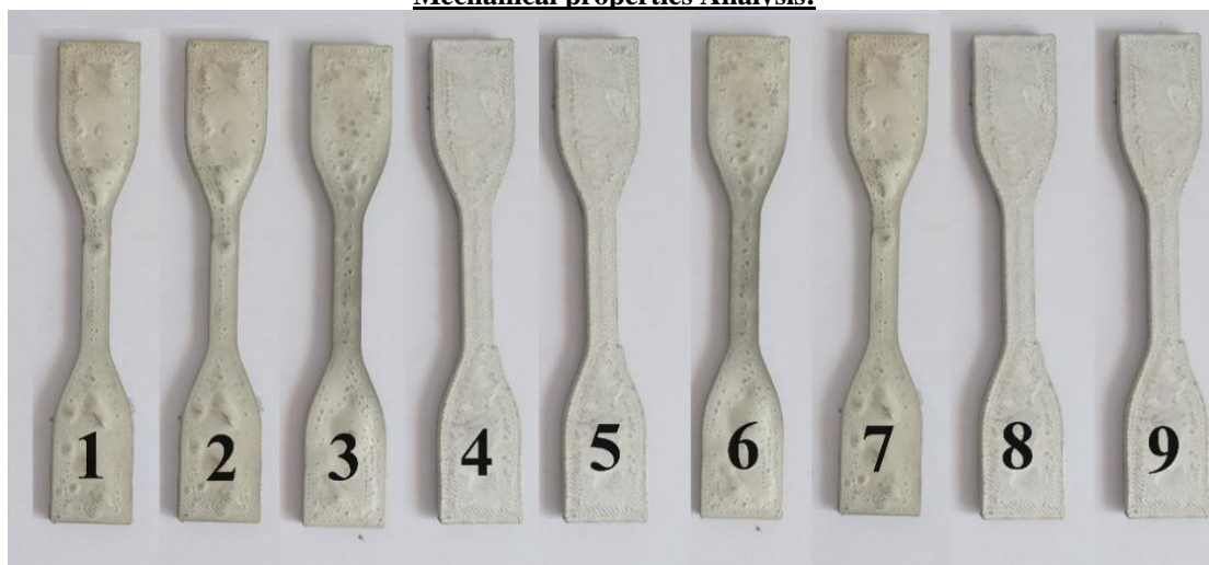
Fig 8: Sintered tensile test specimens printed at different operating parameters
