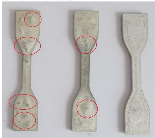
Fig 11: Dimples formation during sintering process
