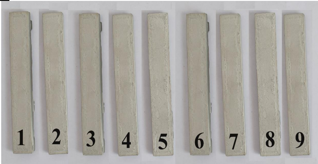
Fig 12: Sintered flexural test specimens printed at different operating parameters
