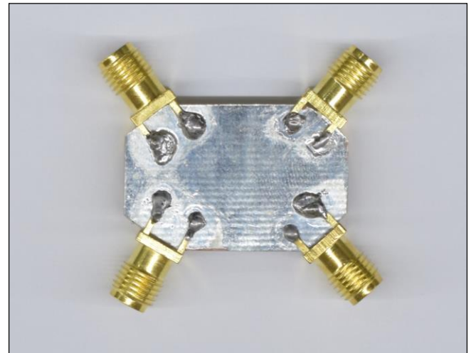
Fig (11): Back side of the module of the proposed distributed branch line coupler
