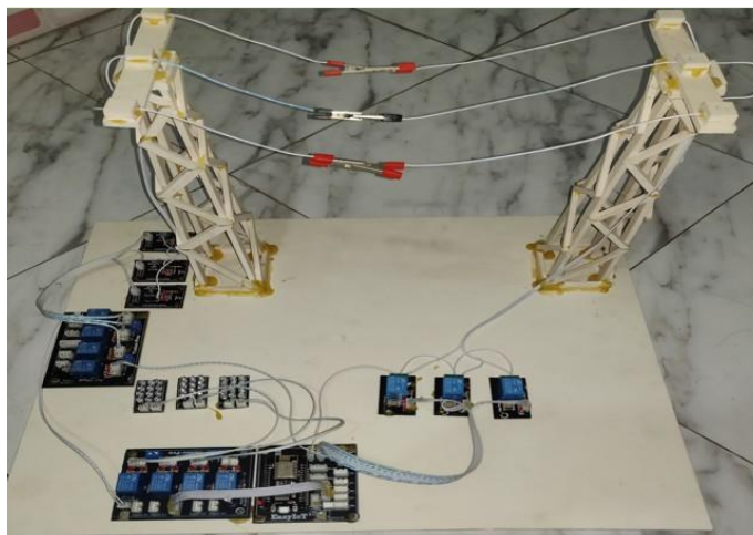
Figure 6: Prototype Design of IOT Based Three Phase Transmission Line Fault Dictation Analysis
