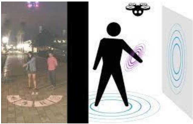
Figure 6: [10]. (Cleared out) User connection with the drone.io menu amid a campus tour. (Right) The drone.io concept permits for different projection spaces including the ground, a divider, or the user's body.
