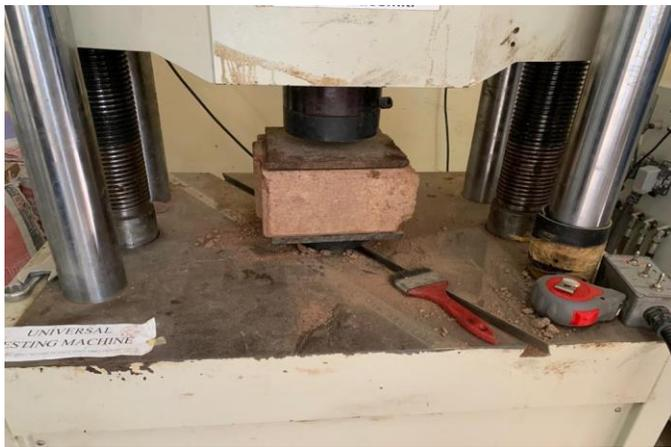
**Fig. 2.** Testing of compressed earth blocks
