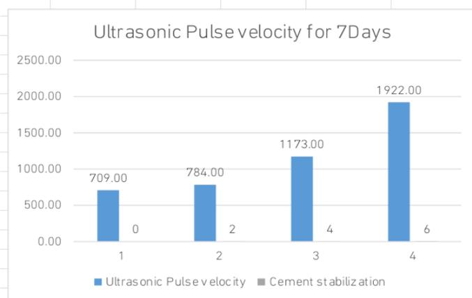
**Fig. 3.** Ultrasonic pulse velocity at 7 days curing
