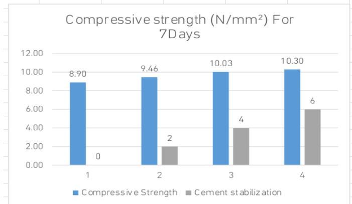
**Fig. 7.** Compressive strength after 7 days curing
