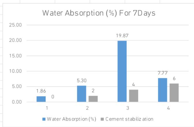
**Fig. 5.** Water absorption after 7 days curing
