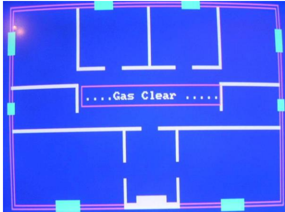
Fig.13 Main Monitoring System of Automatic Gas Leakage Protection
