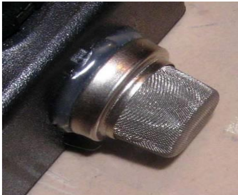
Fig.1 Installation of Gas Sensor
