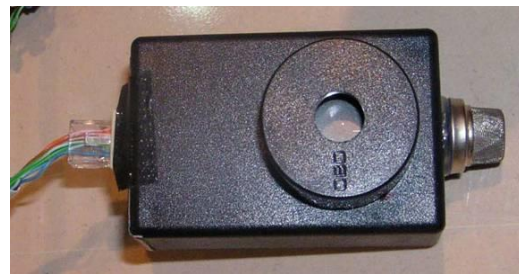
Fig.2 Installation of Speaker with Gas Sensor
