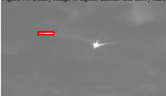
Figure 11. Binary image of fighter aircraft and decoy flares
