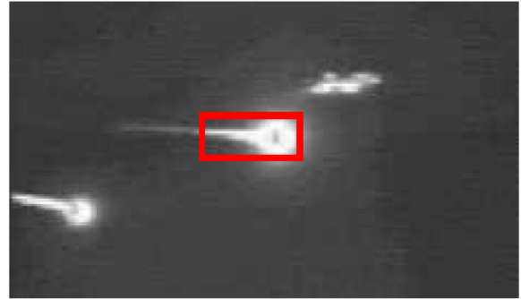
Figure 19. IR radiation emitted by decoy flares compared to aircraft
