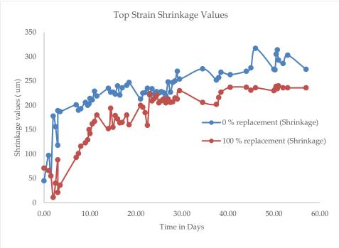
Figure 9. 60- Day Shrinkage Strain Values for the 0 % and 100 % replacement of Conventional aggregate with Tuff Aggregate. The maximum values of 0.000317 mm/m and 0.000236 mm/m for the 0 % and 100 % replacement were measured using shrinkage strain gauges.
