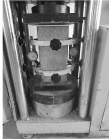
Figure 4. Modulus of Elasticity Testing Equipment undertaken at the Kenya Expressway Project, Nairobi.
