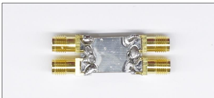
Fig (19): Back side of the module of the lumped-distributed branch line coupler v2
